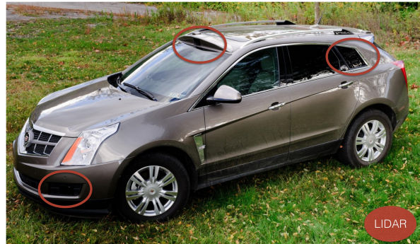
Fig. 1: CMU autonomous vehicle research platform “SRX”
